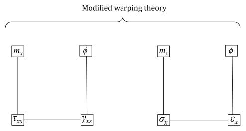
Figure 5: Combined BVP for warping torsion considering both shear and axial strains.
