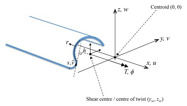
Figure 2: Beam axis system and corresponding displacements.
