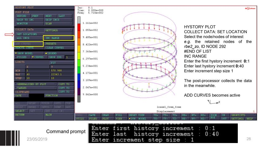
The automatic collection of natural frequencies of the coil (#40 modes) can be done by using HYSTORY PLOT option. These data can usually exported to make the post-processing in a Spreadsheet file, *e.g.* .xls, .xlsx, .ods, ... files.
