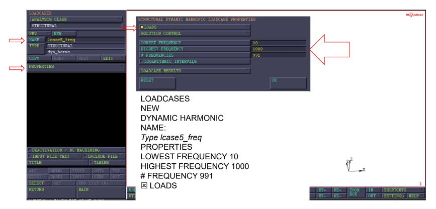
The frequency range that is investigated starts from 10 to 1000 Hz with a discrete step equal to 1 Hz.
