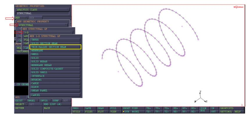
The coil geometric property is defined for thinwalled section beam, where the hollow circular cross section is assessed setting:
