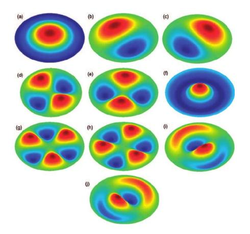
The first 10 mode shapes for a fully clamped circular disk
